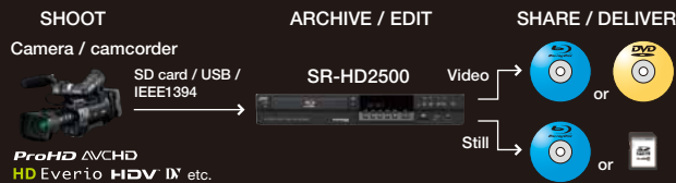
Share HD content #1: Edit and record footage from HD/SD camera to a disc via the HDD and share
